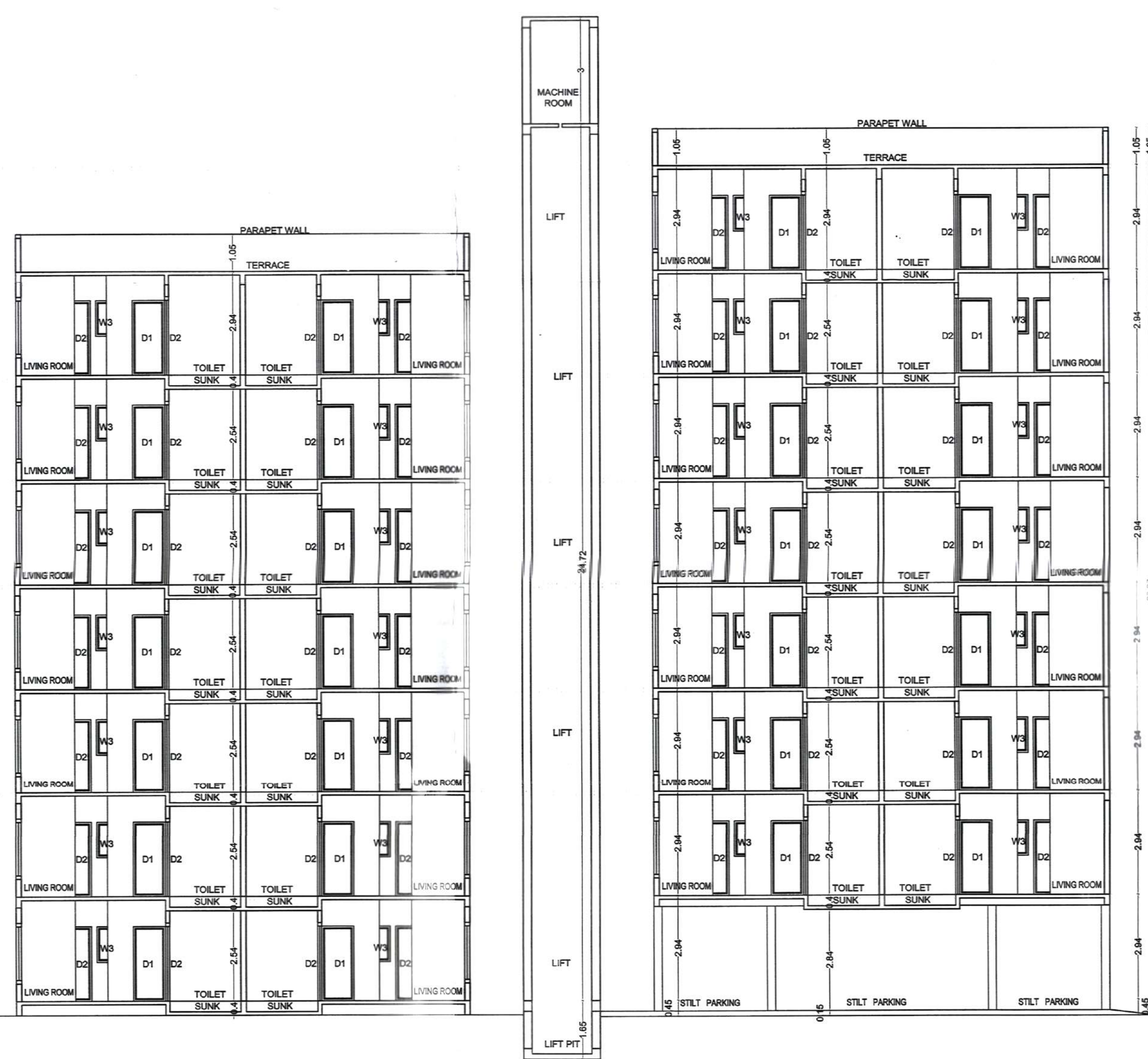
SECTION AT YY SCALE: 1:100 BUILDING - 1
