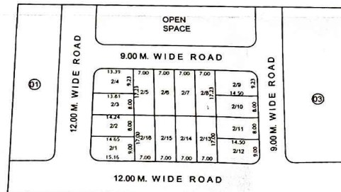
Proposed Sub Division of Plot No. 2 SITE PLAN scale = 1: 1000
