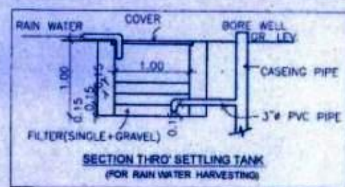
SECTION THRU SETTLING TANK (FOR RAIN WATER HARVESTING)
