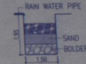
RAIN WATER HARVESTING CHAMBER SECTION
