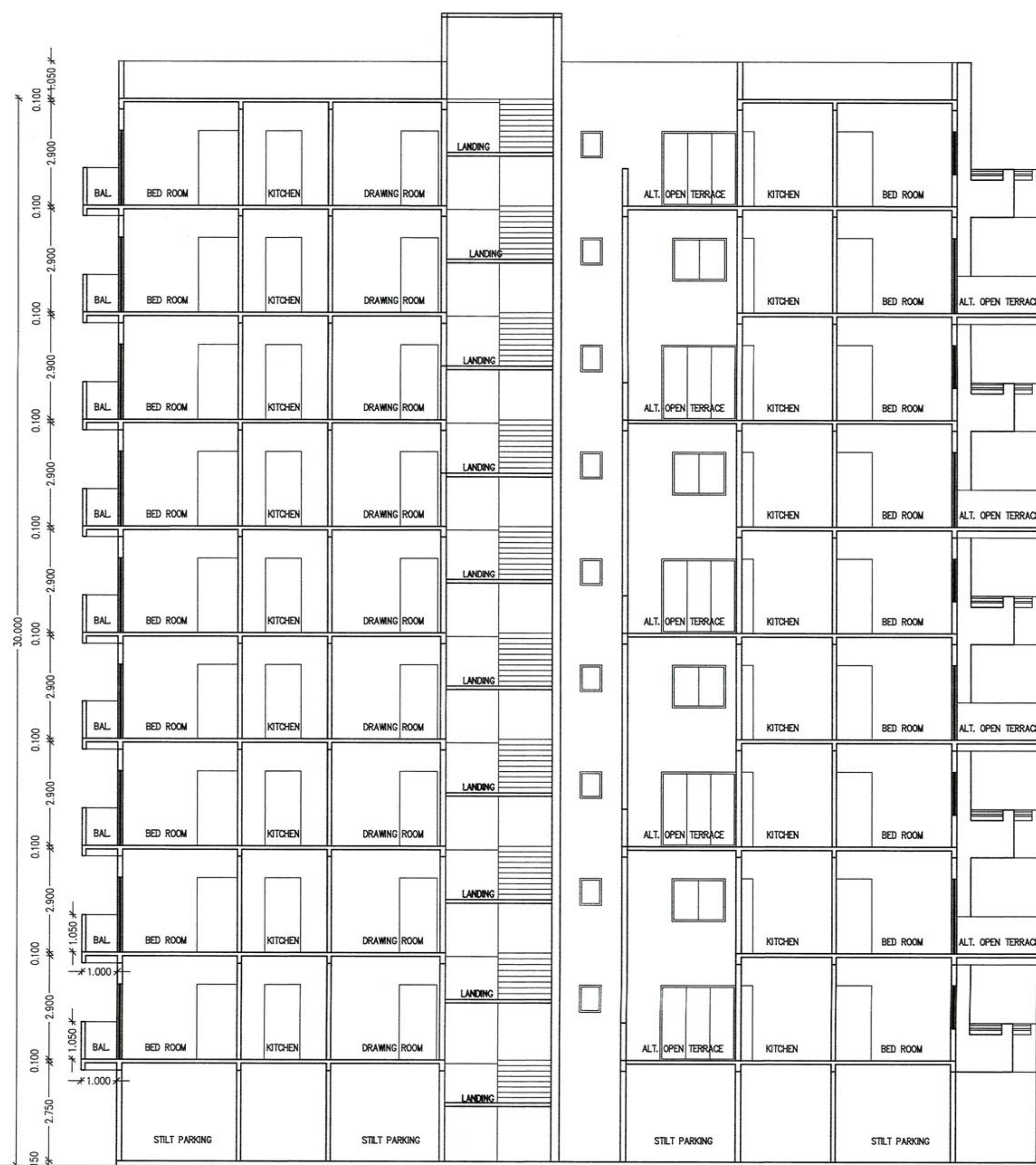
SECTION EE SCALE 1:100 EXISTING WING -B & C
